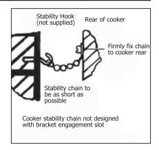
**WARNING:** In order to prevent accidental tipping of the appliance, for example by a child climbing onto the open door, the stabilizing means must be installed.
